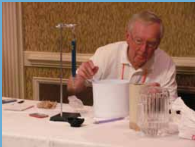
Jim determining the SG of a salt at the Convention
